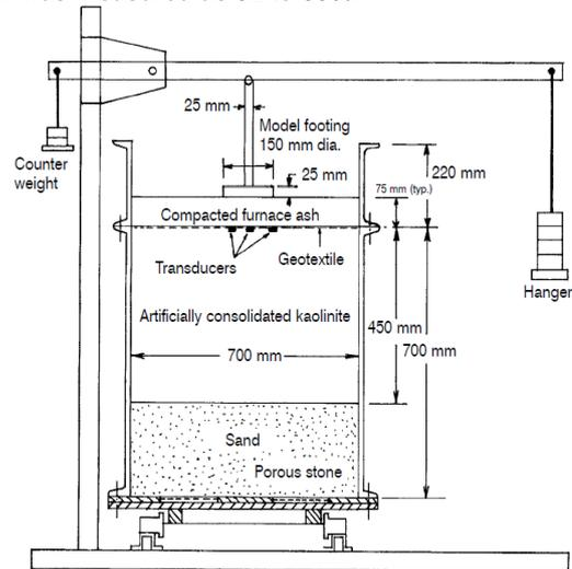
**Figure-1: Test Set-up for the Laboratory Model Footing Test.**
